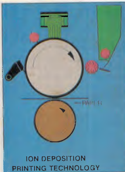
Fig 3 A schematic diagram of an ion-deposition printer. A modulated ion source (top) similar to that in a triode electron tube generates the ions, which are directed onto the drum, forming a latent image. The image attracts toner from the cartridge, which then is pressure-fused onto paper passing between the drum and a pressure roller (Figure courtesy of C.Itoh Electronics)
