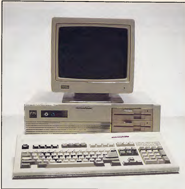
Technology Interface includes the new IBM-style keyboard with 12 function keys, separate numeric and cursor keypads
