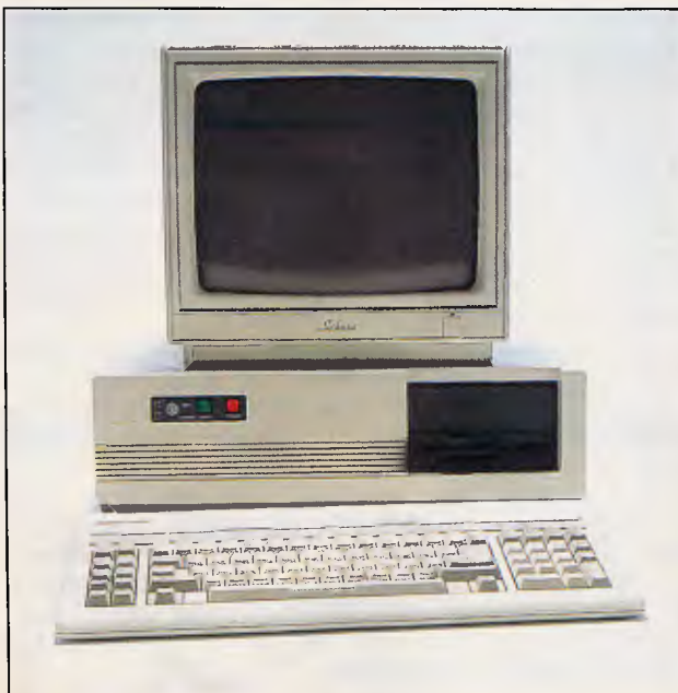
The Rod Irving XT features the Phoenix BIOS 2.27, Microsoft's MS-DOS 3.2 and GW-Basic
